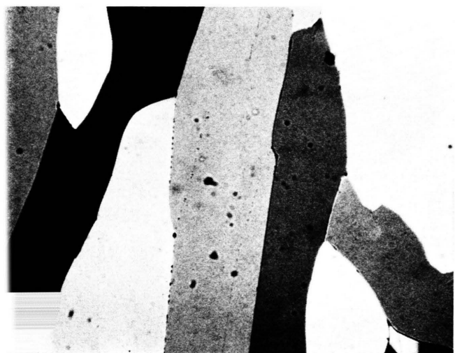
Fig. 2. Mosaic smectic-B texture of (5,5) at 29 °C. Crossed polarizers. Polarizers rotated by 40° on going from a to b. Magnification 80 \times .
