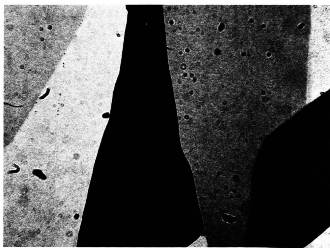
Fig. 3. Mosaic smectic-B texture of (5,5) at 29 °C containing a homeotropic domain (black domain in the center). Crossed polarizers. Polarizers rotated by 20° on going from a to b. Magnification 80 \times .
