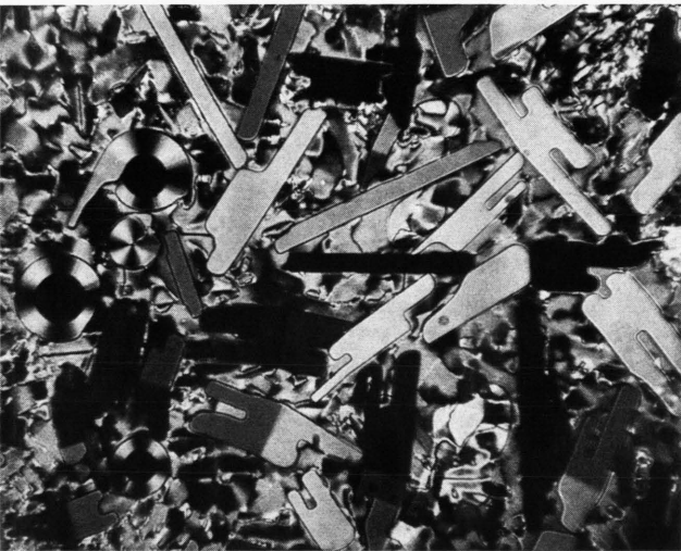
Fig. 5. Smectic-B crystallites growing in the nematic phase of (5,4) at 24.5°. Crossed polarizers. Magnification 80 \times .
