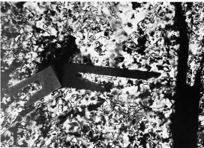
Fig. 6. Individual smectic-B crystallites with sharp edges and split ends growing in the nematic phase of (4,5) at 6.0 °C. Crossed polarizers. Magnification 160 \times .
